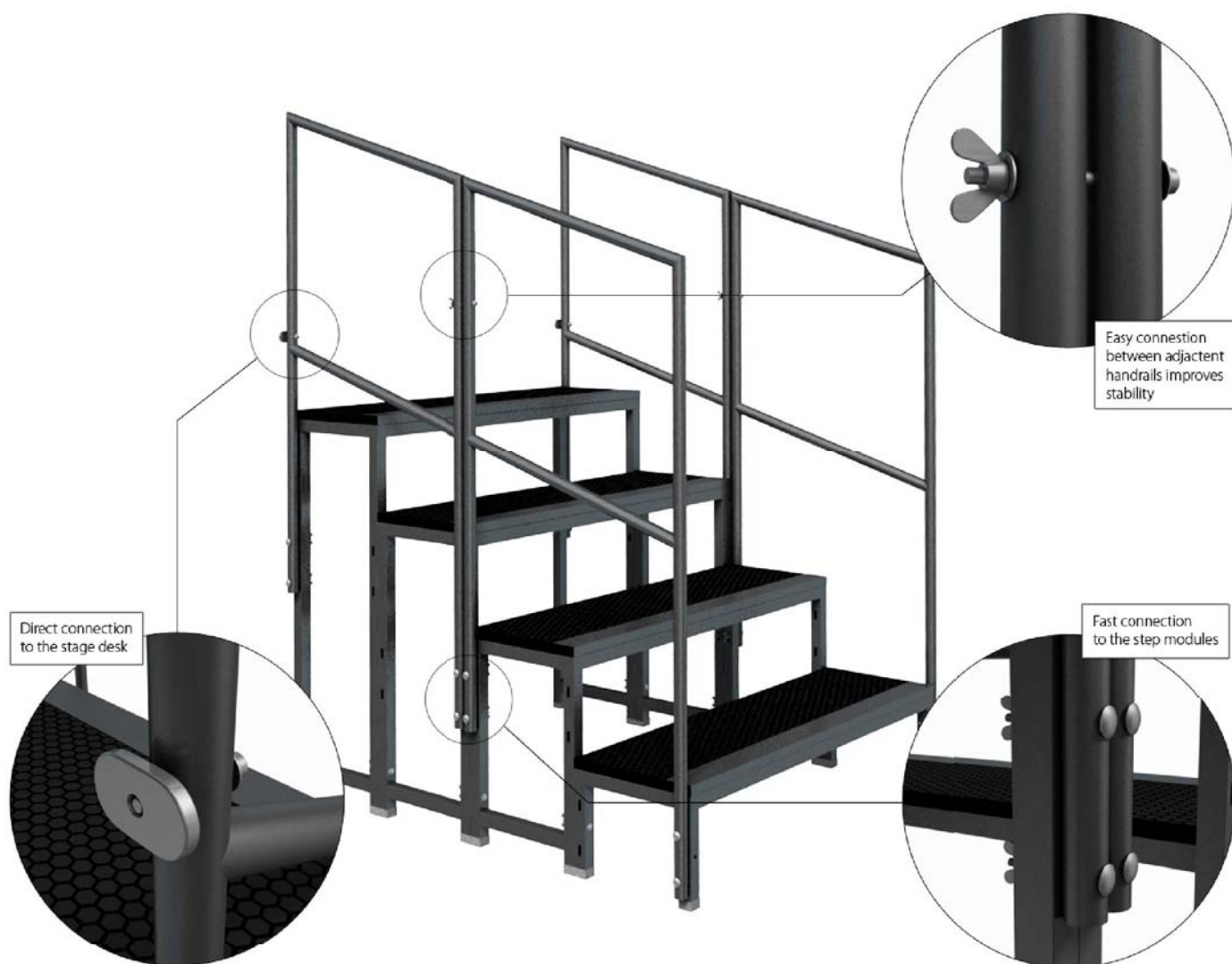
Handrail for modular stairs, assembled on two adjacent steps
